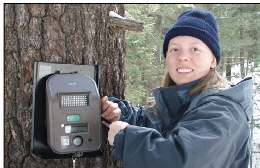
**Approach.** At the Mount Bigelow eddy covariance tower in the Santa Catalina Mountains, and at the Mixed Conifer eddy covariance tower in the Jemez River Basin, we mounted a single overstory “tower-cam” just above the Li-Cor 7500 CO<sub>2</sub>/H<sub>2</sub>O IRGA and three understory “pheno-cams” at heights of 1 m within the footprint of the towers. All four cameras record images hourly.
