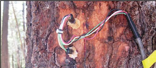
Bark is cleared from installation site. Two 30-mm holes are drilled vertically about 40 mm apart and probes are inserted.
