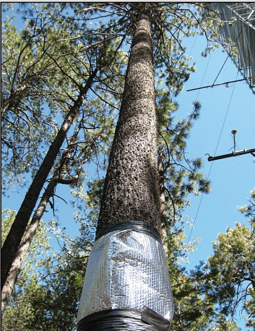
Reflective bubble wrap is wrapped around the tree/sensor, to prevent the sun from causing large local gradients on the stem.
