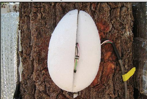
Foam quarter-eggs are taped on either side of the probe needles to protect the sensor wiring and to add thermal insulation.
