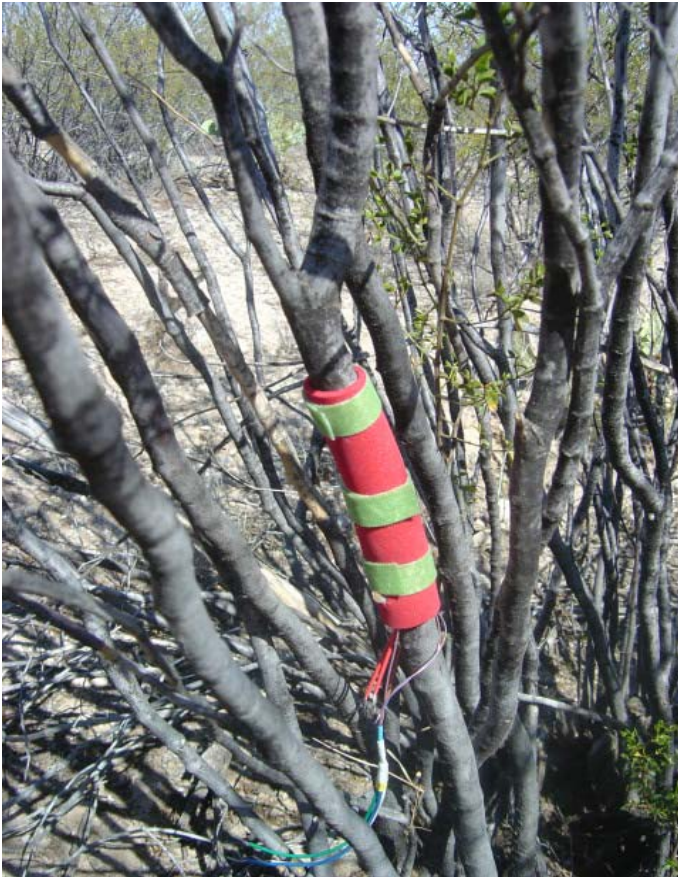
Figure 5: An example of a heat balance sap flow sensor used at the Santa Rita Creosotebush tower site which was constructed in the laboratory. Insulation and weather protection would complete the installation of this instrument. Image by Shirley Papuga.
